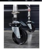
Ensure Castor Wheels are locked in place by pushing down on locking clamp.
